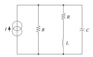
The complex current of the source is  $10e^{j1000t}$ , where j is the imaginary unit. The (angular) frequency is  $\omega = 1000 \text{ rad/s}$ . There are no voltage sources. The corresponding digraph is
