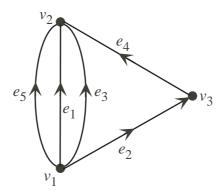
The voltages and currents written as complex exponentials are  $i_k = I_k e^{j1000t}$  and  $u_k = U_k e^{j1000t}$ . In particular, the current source is  $i_5 = s_5 = 10e^{j1000t}$ . We get  $r_k$  from the familiar formulae from electrical circuit analysis:
